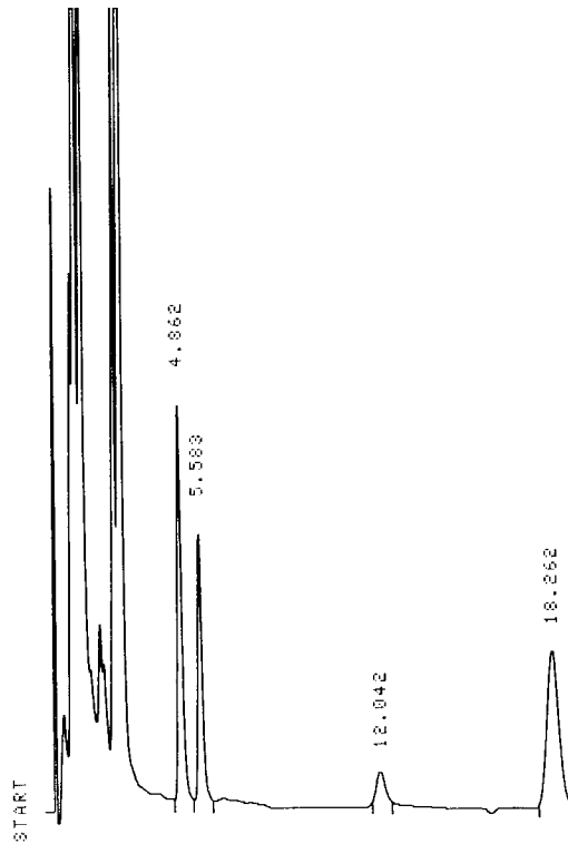
FIGURE 7 Chromatogram of a filtrate of a patient sample; RT: 4.862 CBZ 2.23 [ \mu\text{g/ml} ], 5.583 PT 1.59.
